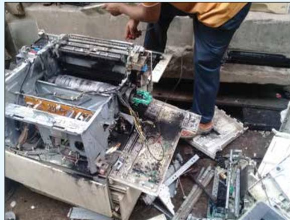
**Photo 5.2 (b): Dismantling Process of Photocopier Machine**
