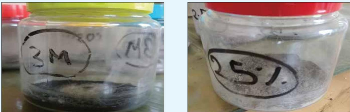
Figure 6.36: Recovered Tin from Different Samples
