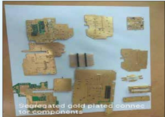
Photo 4.9 (b): Segregated Gold Plated Connector Components
