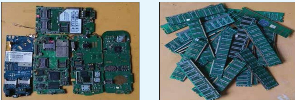
Figure 6.9: Mobile PCBs & RAMs used in Gold extraction
