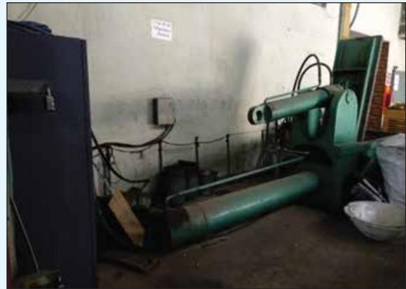
Photo 4.5 (b): Hydraulic Press for Compaction
