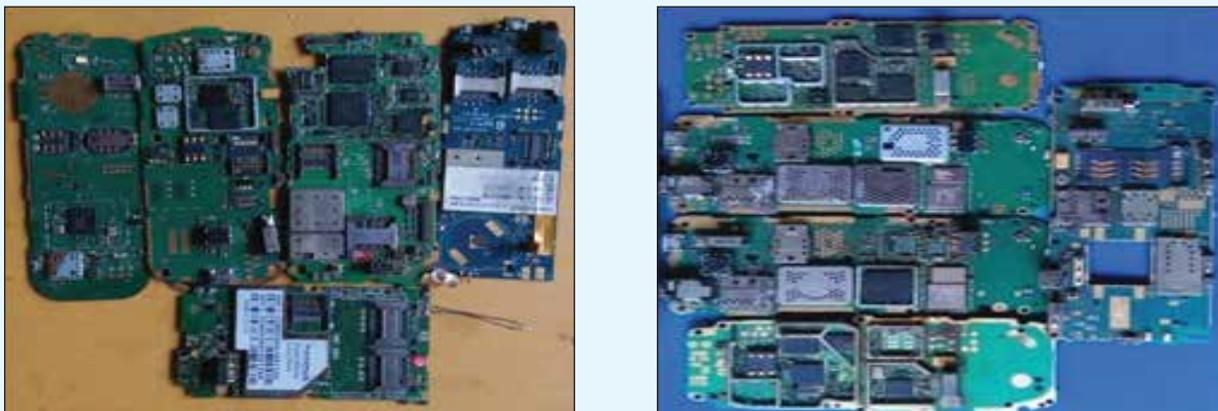
Figure 6.19 Mobile PCBs for Silver Extraction
