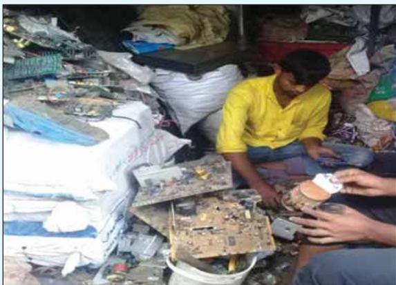
Photo 5.1 (a): Dismantling the Parts from PCB
