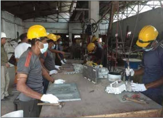
Photo 4.8 (a): Manual Dismantling Process
