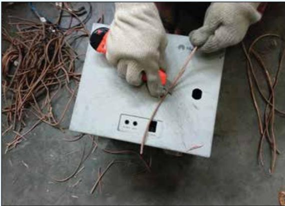
Photo 4.5 (a): Manual separation of Copper Wires
