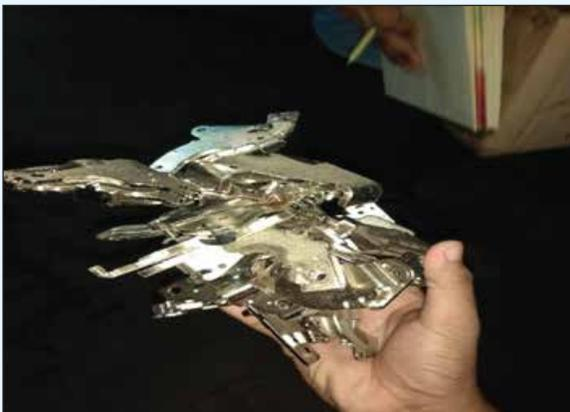
Photo 4.5 (c): Rare Earth Magnets Used in Hard discs
