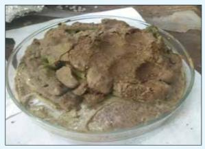
Figure 6.13: Brown solid mass after drying at 100 degrees for 24 hours
