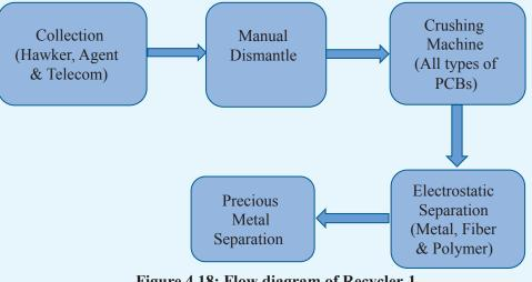
Figure 4.18: Flow diagram of Recycler-1
