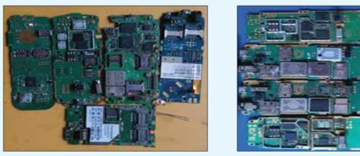
Figure 6.19 Mobile PCBs for Silver Extraction
