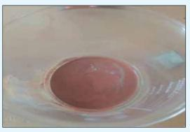
Figure 6.32: Dried Cu Powder from Graphite Cathode
