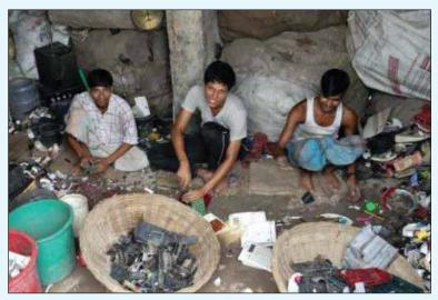
Figure 2.18: Workers Manually Dismantling Scrap Electronics (ESDO, 2010)
