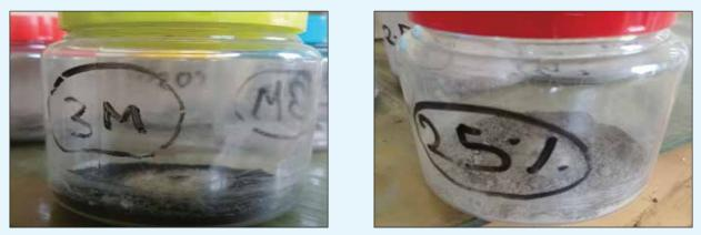
Figure 6.36: Recovered Tin from Different Samples
