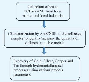
Figure E.3: Methodology for value metal recovery from E-waste
