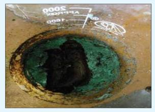
Figure 6.12: Brown Mud with Bluish Green Precipitate Layer
