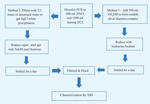
Figure 6.20: Flow Chart of Ag Extraction from PCB
