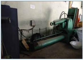
Photo 4.5 (b): Hydraulic Press for Compaction
