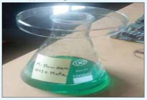
(a) (b) Figure 6.29: (a) Mobile PCBs (b) Metal Powder Dissolved in Acid +  ${\rm H_2O_2}$
