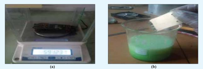
Figure 6.28: (a) Weighing of the PCB in Electric Balance (b) Dissolving PCB in Acid Solution
