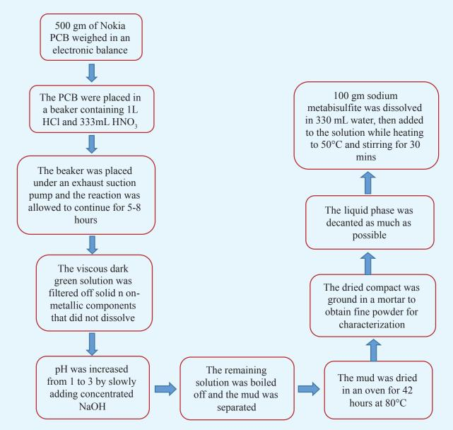
Figure 6.10: Flow chart of the Gold Extraction Process
