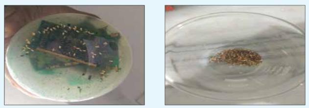
Figure 6.18: Gold Separation by Ultra-sonication with DMA
