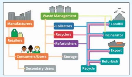
Figure 2.17: E-waste Recycling Process Flow (Schluep et al., 2009)
