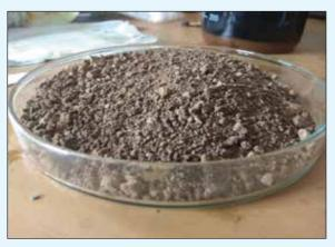
Figure 6.14: Brown powder mass after grinding
