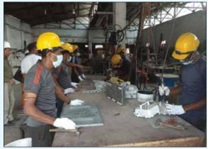
Photo 4.8 (a): Manual Dismantling Process
