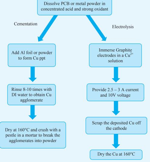
Figure 6.27: Flow chart of the different processes of Cu extraction
