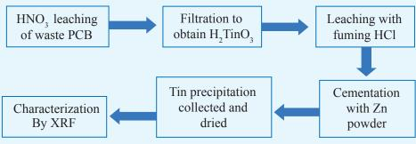
Figure 6.35: Flow Diagram for Tin Extraction
