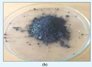
Figure 6.22: (a) AgCl Precipitate at the Bottom (b) Solid Powder for Characterization
