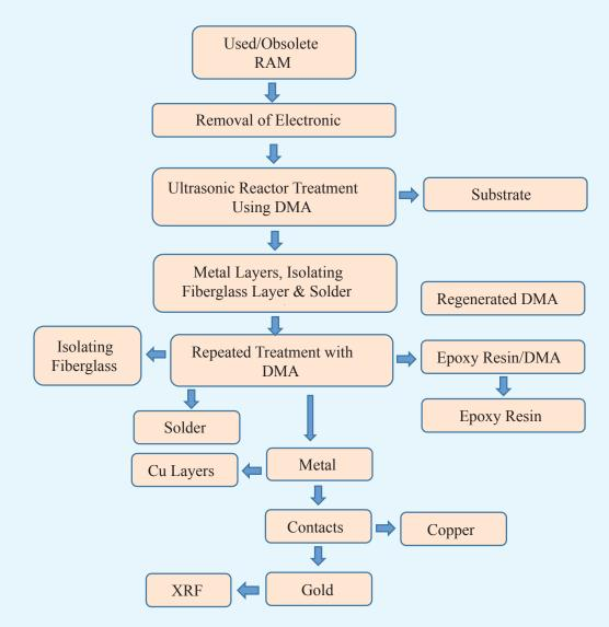
Figure 6.16: Process Flow of Gold Separation from RAM by DMA Treatment
