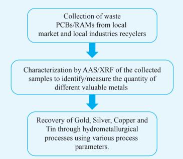
Figure 3.5: Methodology Used for Value Metal Recovery from E-wastes
