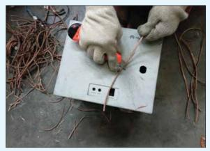
Photo 4.5 (a): Manual separation of Copper Wires
