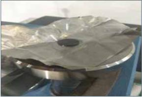
Figure 6.24: Silver Tablet Sample for XRF Analysis
