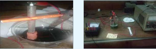
Figure 6.31: Electrolysis and Cu Deposits on Cathode
