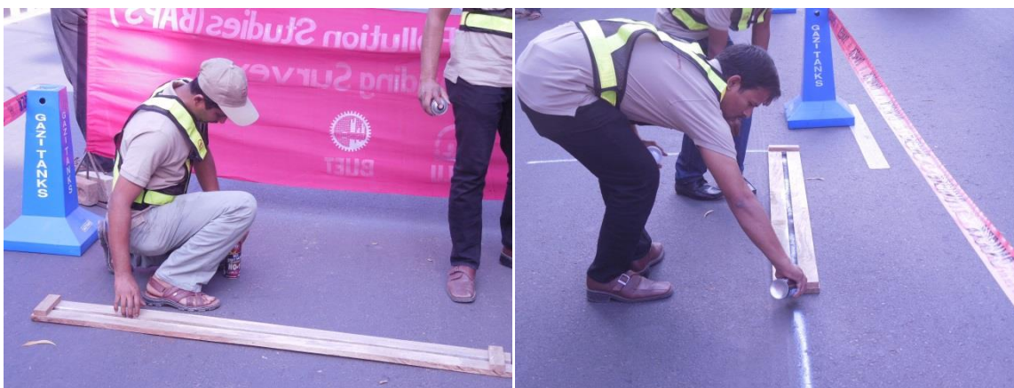
Figure 6: Marking on the road surface for road dust collection
