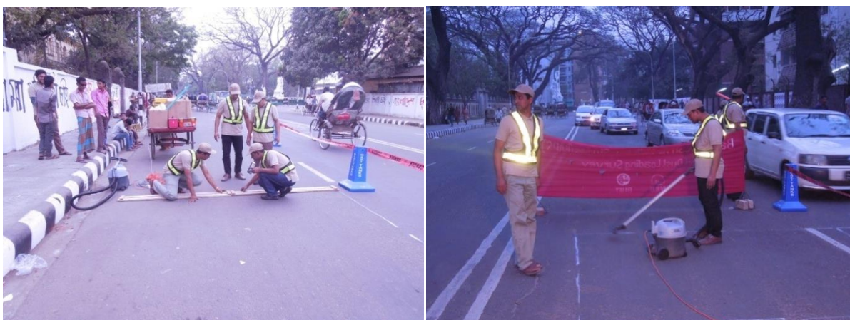
Figure 7: Collecting road dust with high efficiency vacuum cleaner
